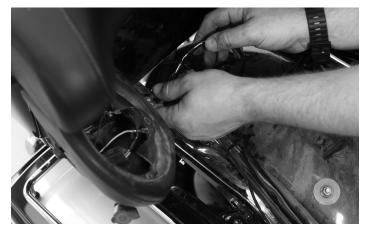
Connect the factory speaker connectors to the male spade terminals on the new harness. Connect the new harness to the Rockford speaker terminals using the female connectors.
