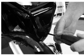
After the screws are removed, use your socket or ratcheting wrench to unbolt the turn signal brackets.
