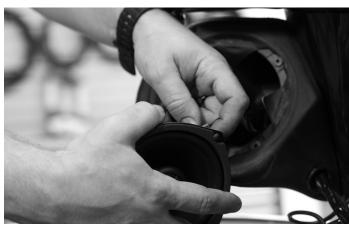
Once all of the terminals are connected, insert the new speaker and factory grille so you can fasten to the speaker pod.
