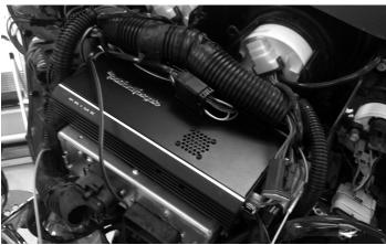
Models equipped with the communication module, installing the supplied rubber foot to the bottom side of the amplifier is required.
