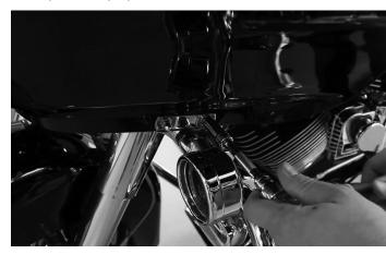
Pull the fairing toward the front of the bike and up to release it from the fairing mounts. Unplug headlight harness and set fairing aside.
