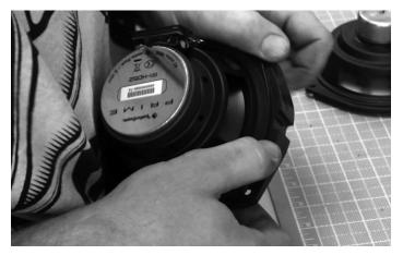
NOTE: You can insert the one side of the speaker into the assembly and use a flat bladed screwdriver or pry bar to gently pry the grille onto the speaker for a tight fit. Be sure to orientate the speaker with the terminals up.
