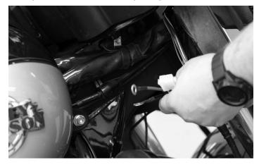
Routing the new wire harness along with the factory harness is recommended. Be sure to zip tie the harness together for a clean, tight fit.
