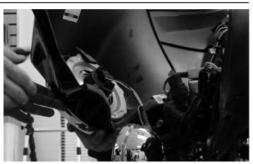
You will need to disconnect the harness from the headlight to completely take the fairing off of the motorcycle.
