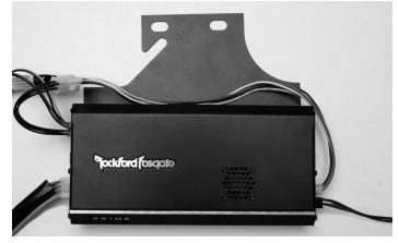
Mount the bracket to the brake side turn signal bracket. Once the amplifier is mounted, you can now wire up the speakers.
