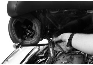
Connect the additional harness and route the speaker wires into the speaker pods.
