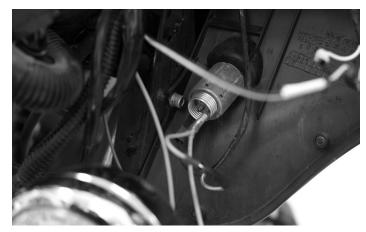
NOTE: When routing your wires, be sure to avoid sharp edges which may cause damage to the wiring harnesses. Any extra wiring should be zip tied up and out of the way of components.
